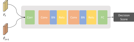
Fig. 3. Scheduler network. The output feature map of the correlation layer is followed by two convolutional layers and a fc layer with a 2-way softmax.
